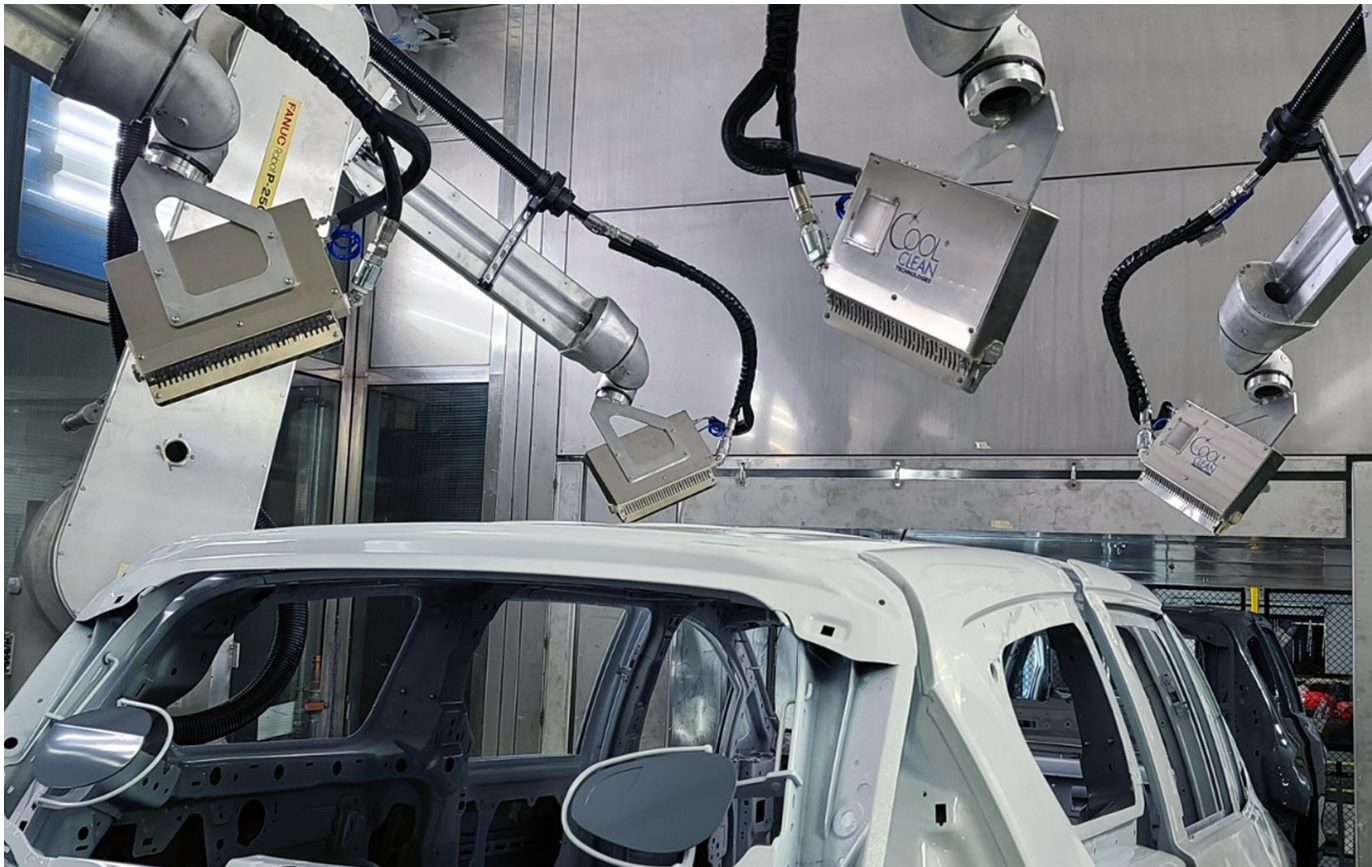
Automated CO2 Cleaning for Car Body
